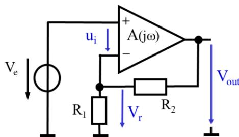
$$V_r = \frac{V_{out}}{R_1 + R_2} R_1 = V_{out} \left( \frac{R_1}{R_1 + R_2} \right)$$
