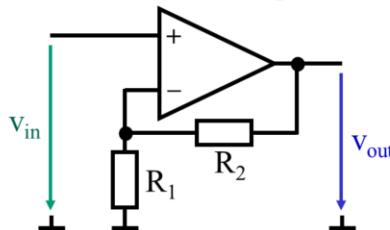
$$\begin{aligned} R_1 &= 1 \text{ k}\Omega \\ R_2 &= 10 \text{ k}\Omega \\ \text{AO: } &\text{GBW} = 1 \text{ MHz} \end{aligned}$$
